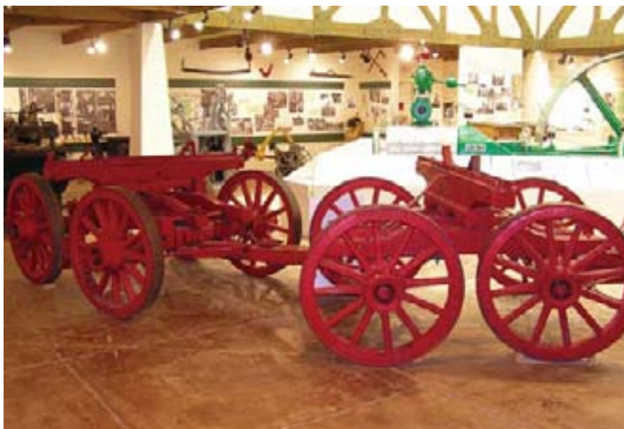
This eight-wheeled logging wagon was designed to turn corners.
