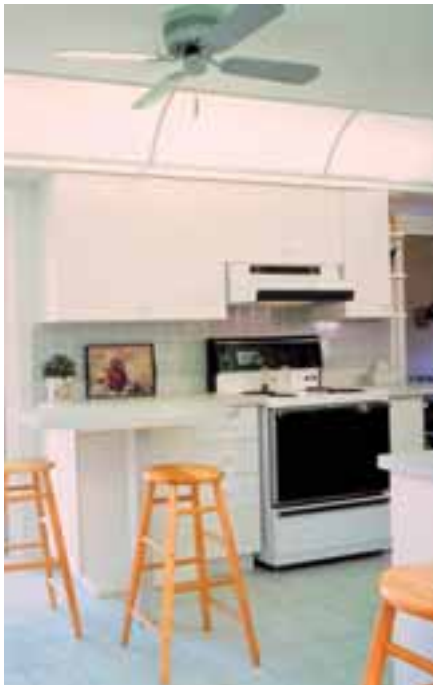
Ceiling fans help reduce air-conditioning and heating use.
