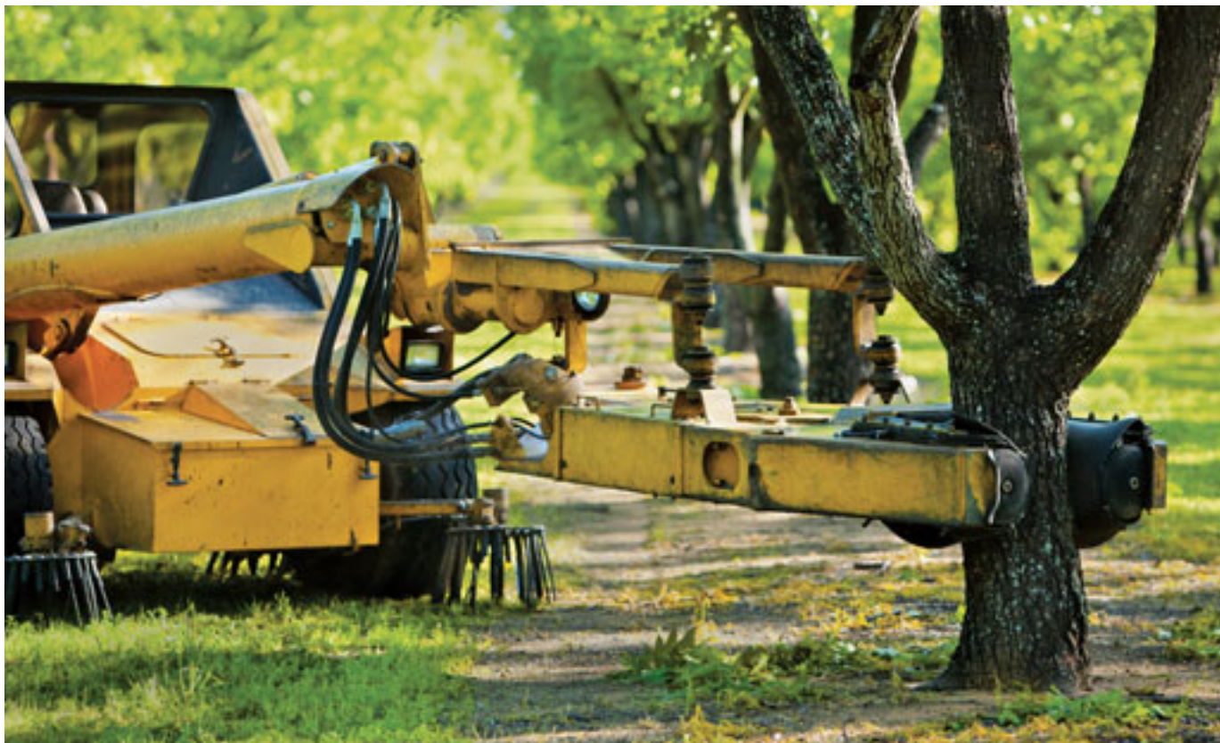
Hydraulic pinchers grab on to a pecan tree trunk and shake the nuts down.
