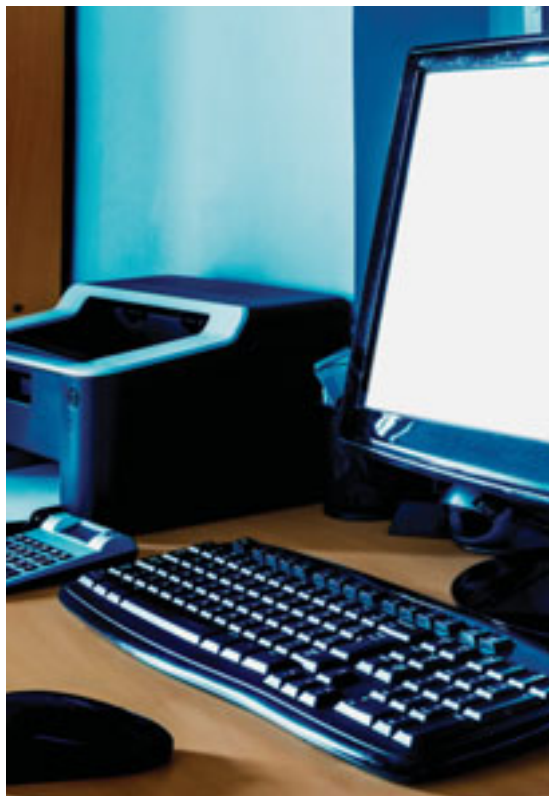
Moving computers, printers and chargers to the same area makes them easy to control with a single power strip.
